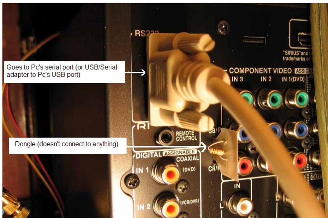
5) Plug in the Onkyo receiver’s power chord. All lights should be off, including the standby light. If standby light is on, unplug Onkyo receiver’s power chord, check connections, and plug receiver’s power back in, being sure all lights are off.
