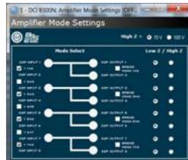
One HF tuning and one LF tuning would be used for each bi-amplified speaker. After configuring two channels for “bi-amplified” configuration using the MODE icon, select the appropriate LSR705i, LSR708i or M2 HF and LF speaker tuning for the amp channels in the bi-amplified pair. Exit and Save your file.
