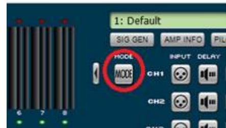
On the mode settings, select the “Y” configuration for the amp channels you wish to bi-amp. As an example, this picture shows a DCi8300 configured for bi-amp tunings
